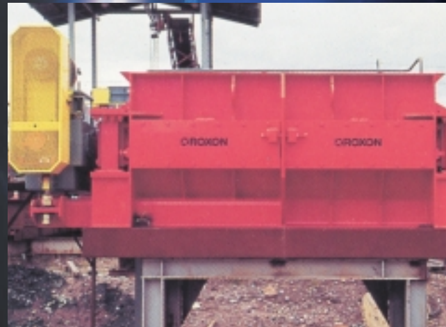
CUMERA GEAR DRIVE ON A WOOD CHIPPER
