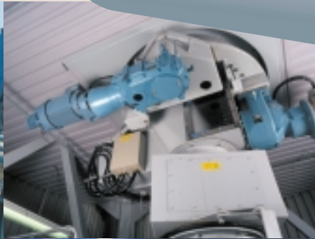
CUMERA GEAR FOR ROTATING DRIVE OF A SCREW UNLOADER
